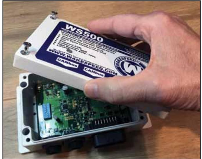
Figure 3 — Removing regulator lid
