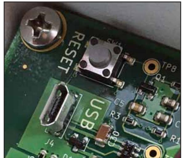
Figure 7 — Micro USB connector & reset button
