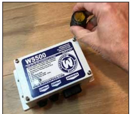
Figure 2 — Unscrewing regulator lid
